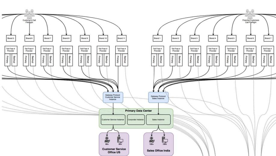
Figure 1. Example of a phone system diagram proposal I created to upgrade call capacity and minimize system downtime
